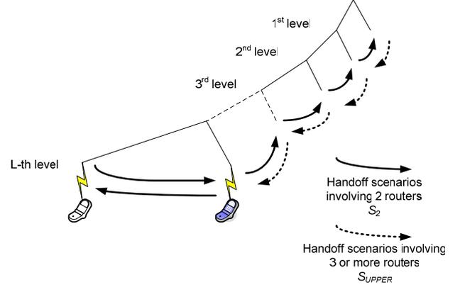
**Figure 14. Worst case scenario for unbalanced hierarchy of routers in which  $S_2$  is minimized**
