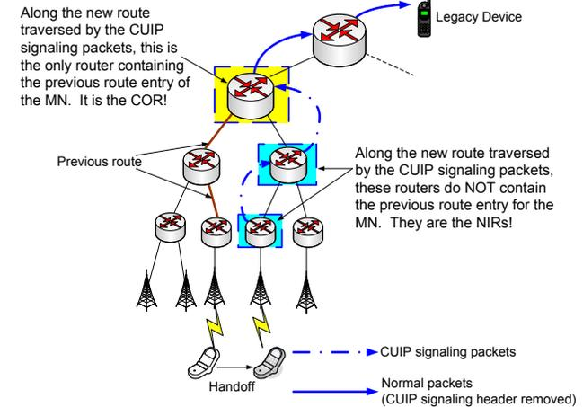
Figure 5. Illustration of the COR self-identification algorithm
