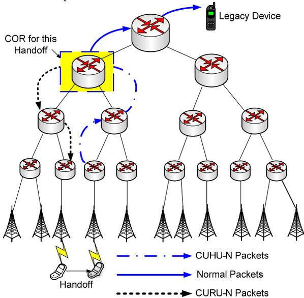
Figure 7. Basic idea of CUHU mechanism
