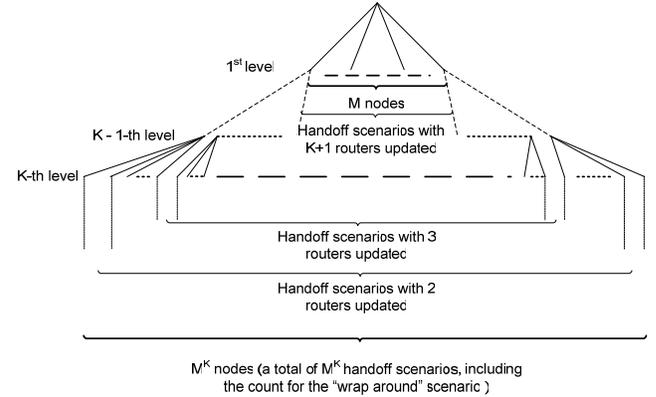
Figure 12. Derivation of  $E[N]$  under a 1-D balanced hierarchical tree structure
