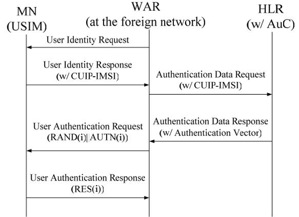
Figure 10. Authentication mechanism in CUIP based Wireless Access Network
