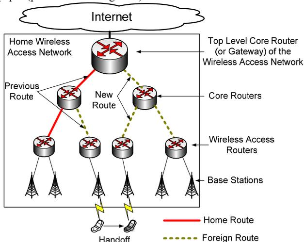
**Figure 2. A sample wireless access network**
