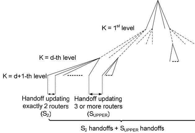
**Figure 13. Derivation of  $E[N]$  under a 1-D unbalanced hierarchical tree structure**
