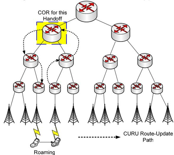
**Figure 6. Basic idea of CURU mechanism**
