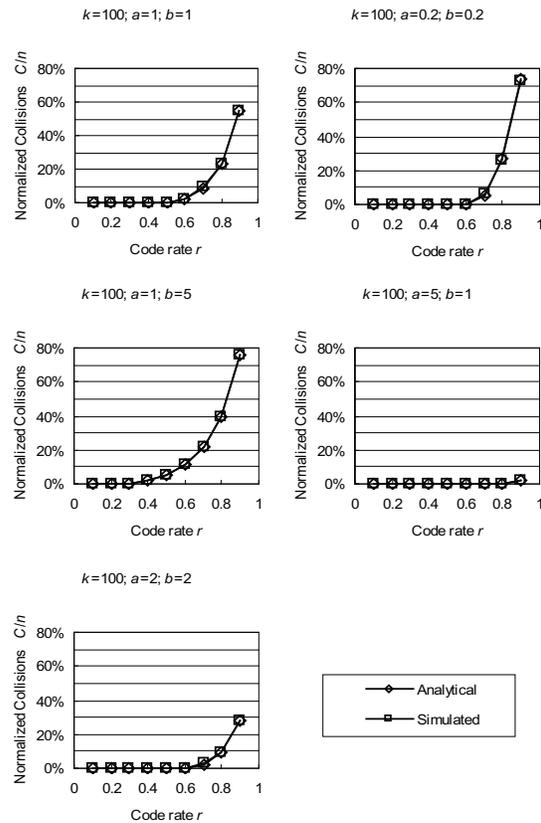
Fig. 9. Analytical and simulated average collisions against the code rate  $r$  for number of peers  $k=100$  with respect to different shape parameters  $a$  and  $b$ .
