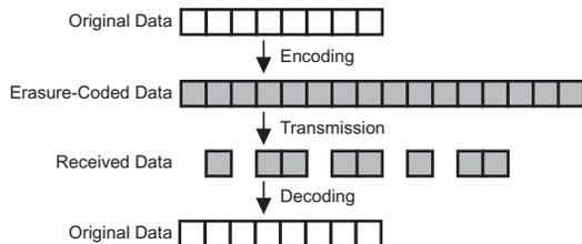
Fig. 1. The process of the erasure-correction coding.
