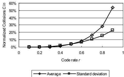
Fig. 11. Trace-driven simulated average collisions against the code rate  $r$ .
