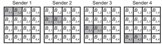
Fig. 5. Peers transmitting the encoded data blocks according to DPRS.
