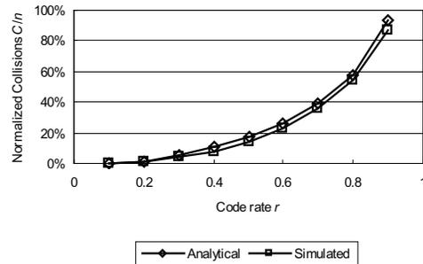
Fig. 10. Analytical and trace-driven simulated worst-case collisions against the code rate  $r$ .
