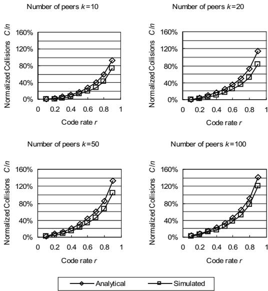
Fig. 6. Analytical and simulated worst-case collisions against the code rate  $r$ .
