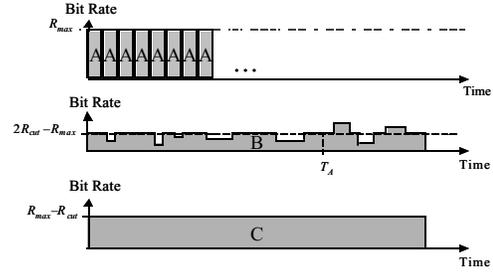
**Figure 3. The three types of multicast channels in the Slice-and-Patch algorithm.**
