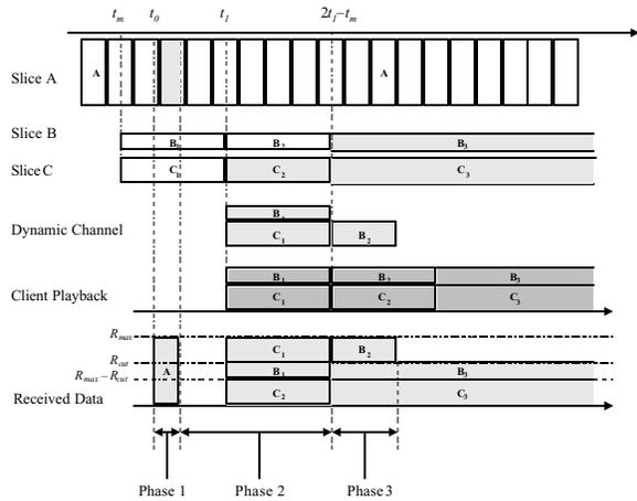
**Figure 4. The three-phase patching process in the Slice-and-Patch algorithm.**
