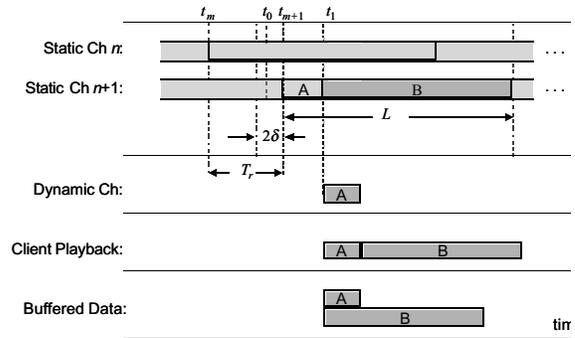
**Figure 1. The patching process in the super-scalar video-on-demand system supporting CBR video.**
