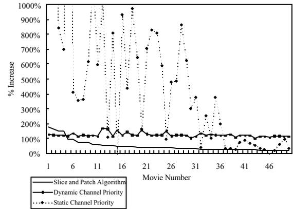
**Figure 5. Percentage of latency increases over CBR-based system for 50 different videos.**
