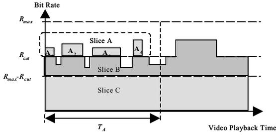
**Figure 2. Video slicing in the Slice-and-Patch algorithm.**
