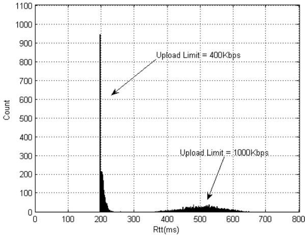
Figure 4. Comparison of RTT distributions at low and high upload data rates
