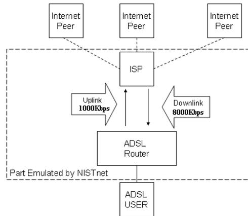
Figure 1. A P2P host running behind a bandwidth-asymmetric network
