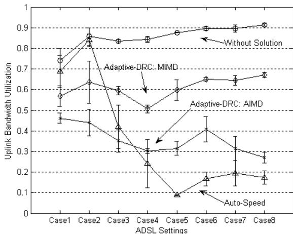
Figure 6. Comparison of uplink bandwidth utilizations
