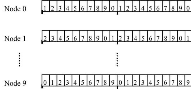
**Fig. 3.** Transmission schedules generated by the Staggered Scheduling algorithm
