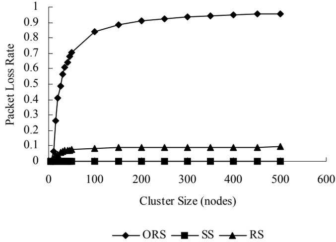
Fig. 4. Comparison of packet loss rate versus cluster size for ORS, SS, and RS
