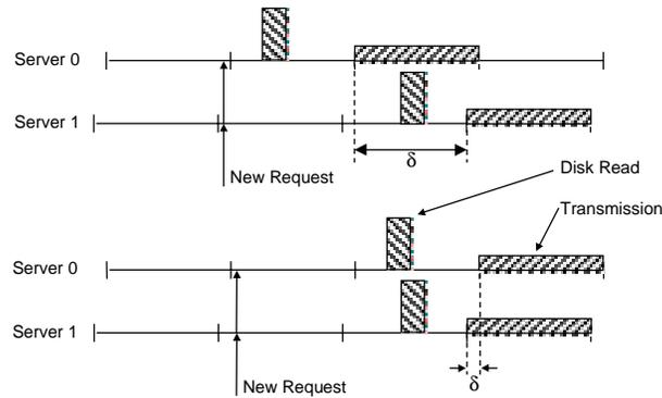
*A small clock jitter can lead to a big transmission jitter!*
