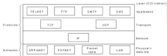
*This is a protocol stack conforming to the TCP/IP reference model.*
