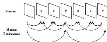
Three types of frames: intra pictures (I frames), predicted pictures (P frames), and bidirectionally interpolated pictures (B frames).
